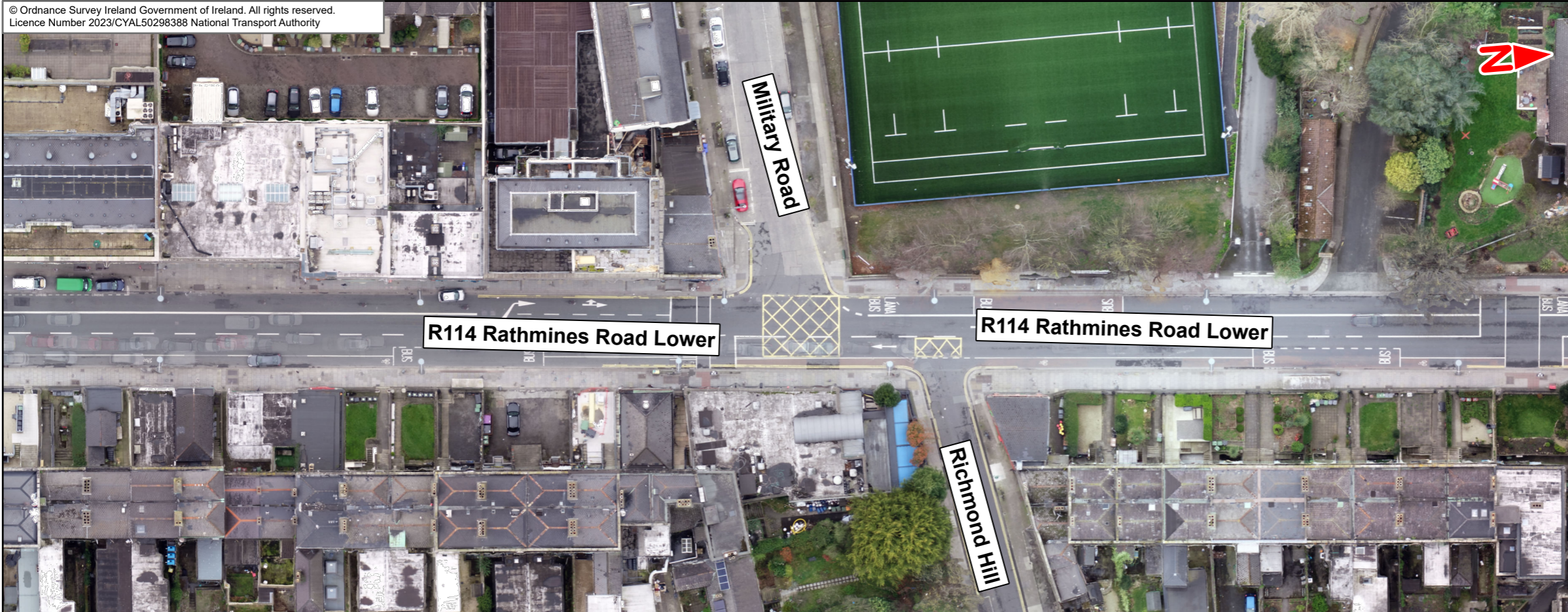
A) R114 RATHMINES ROAD LOWER / MILITARY ROAD / RICHMOND HILL STAGGERED FOUR-ARM PRIORITY JUNCTION
