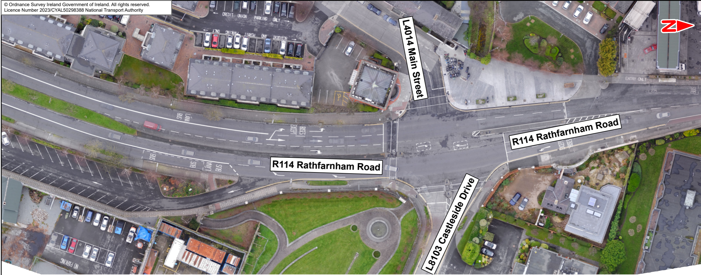
A) R114 RATHFARNHAM ROAD / L8103 CASTLESIDE DRIVE / L4014 MAIN STREET FOUR-ARM SIGNALISED JUNCTION
